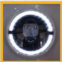
ROUND SHAPE DRL'S PLACED NEATLY IN HEADLIGHT, FOR BETTER NIGHT VISUAL APPEARANCE LED BULB WITH PROJECTOR COVERING WITH CRYSTAL CLEAR GLASS.
